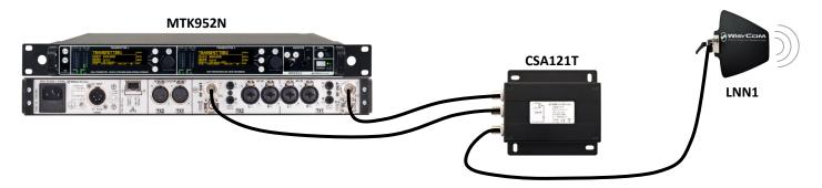
Connecting CSA121T, MTK952N automatically recovers the combiner loss increasing the output power of the transmitter
